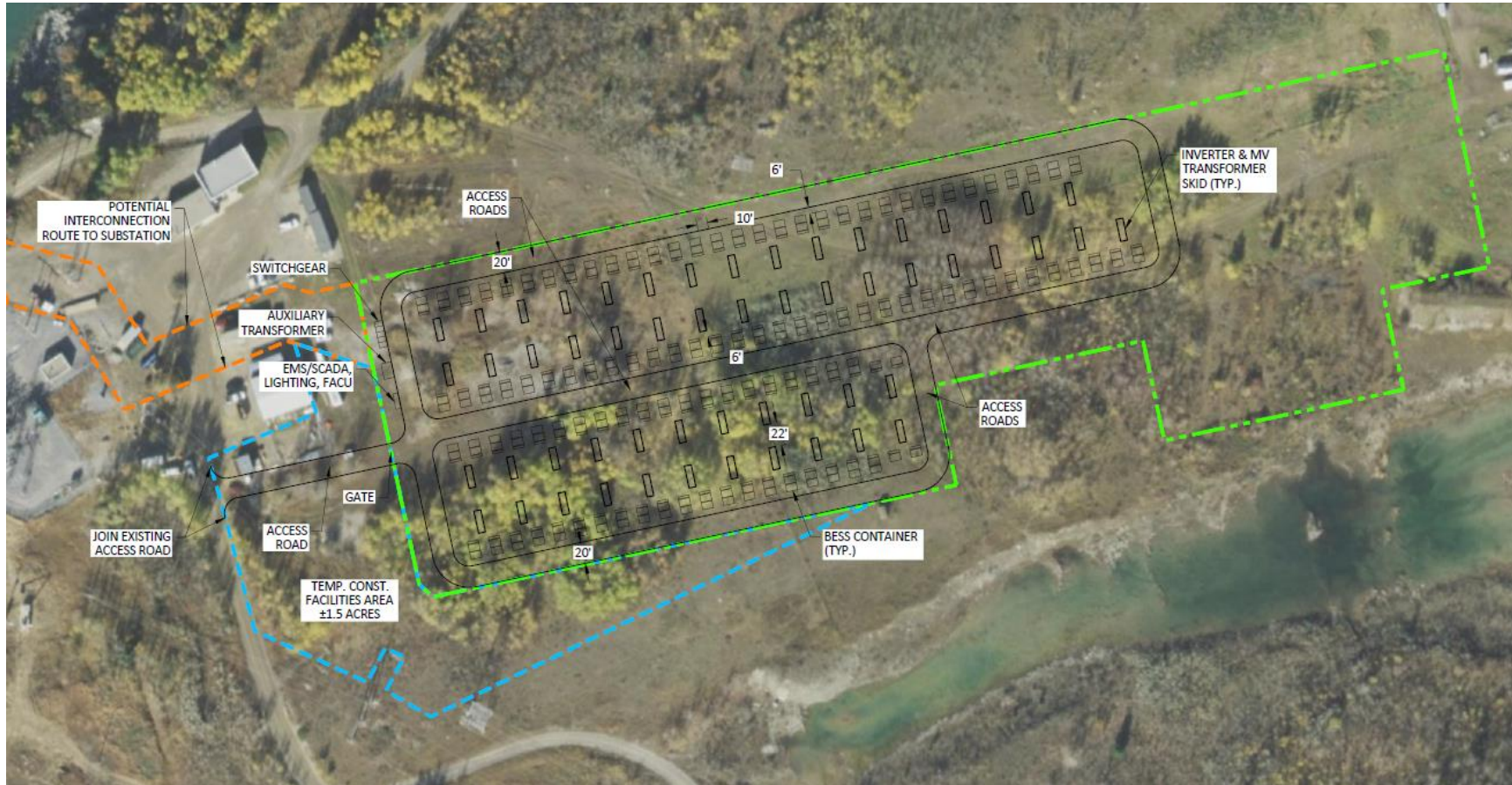
Figure 3 Project plot plan indicating proposed preliminary Vendor B equipment site plan.
